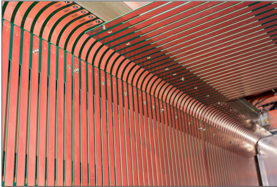
FIG. 9: A photo of the 35 ton LBNE prototype field cage.
