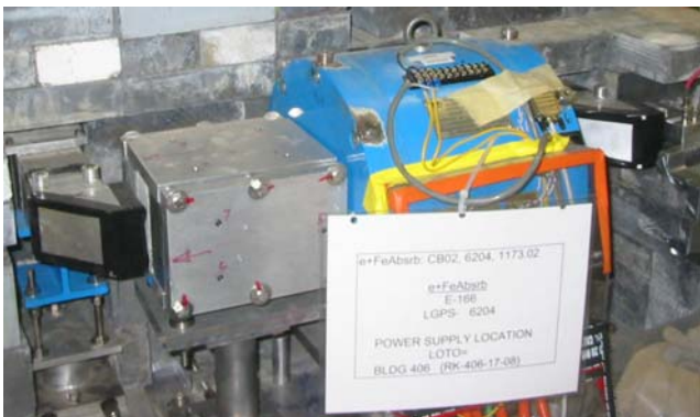
Figure 7: The photon transmission polarimeter during installation. The blue object is the iron-core solenoid whose magnetization is reversed periodically.
