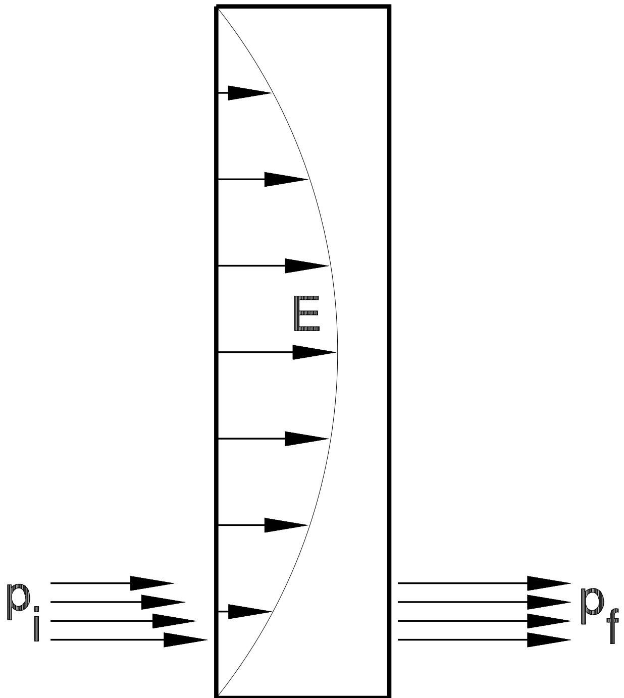
The muon pass through the cavity wall at a momentum dispersion point well off the cavity axis.
