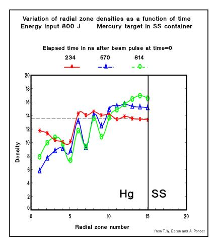
Hydrodynamic calculations of shock waves in a cylindrical mercury target encased in a stainless steel tube using the REXCO code
