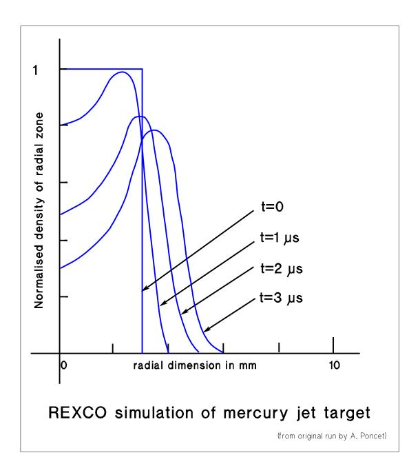
Early simulation of the radial zone density variation in a mercury jet target in which 1 kJ of beam energy is deposited at time zero. The target radius is 3 mm, the length 50 mm and the beam radius (uniform density) is 0.5 mm.
