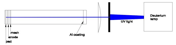
The deuterium lamp light shines on both the Al-coated window and on the solder-coated pad plane, and photoelectrons are emitted from both.
