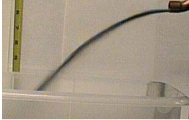
Figure 4: A horizontal jet of 325-mesh tungsten powder after falling 1.5 m inside a 1.25-cm-diameter tube with a 3-cm-radius bend of 90^\circ at its bottom.
