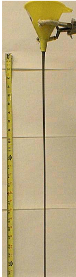
Figure 3: A vertical jet of 325-mesh tungsten powder as poured through a plastic funnel of 1-cm-diameter aperture.
