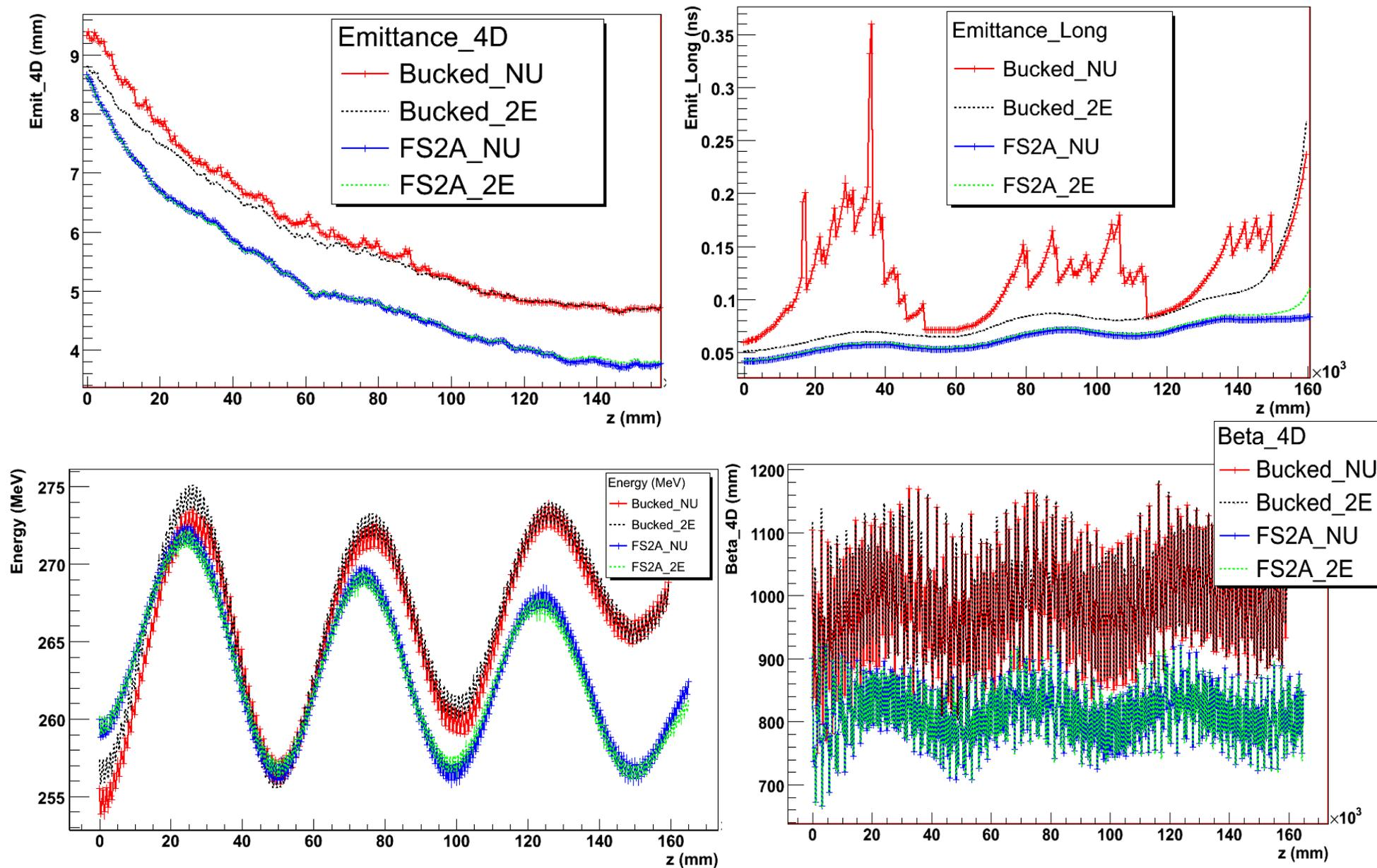
Note that although both beams should start with same  $\langle E \rangle = 254.65$  (i.e. 232 MeV/c), there is a small difference at the energy start point between FS2A and Bucked. Also different start point at Emit4D and EmitLong. This is due to the Beta4D difference.
