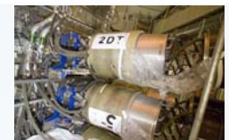
PINI NBI at JET tokamak
