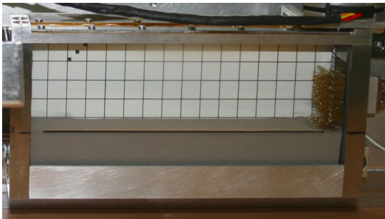
1- Resettable trough with 45um grains
