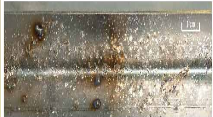
Figure 5. Damage observed on the inside of the vacuum chamber, on the side opposite to the beam impact. Molten material has been projected across the chamber and has condensed in droplets on the other wall.
