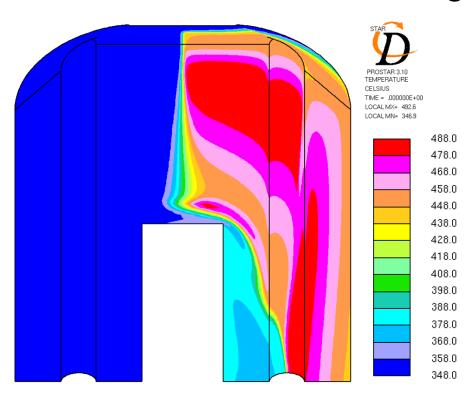
The beam is scanned on the top surface to distribute the power deposition on a channel 12cm and 30cm deep
