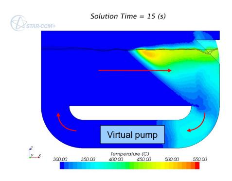
Temperature field on the symmetry plane
