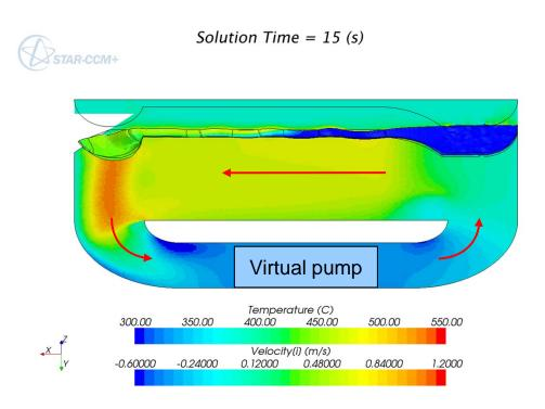
Temperature on the free surf. and velocity magnitude on symmetry plane
