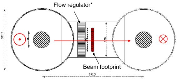
PDS-XADS target module sketch with flow direction and transverse section with beam deposition area
