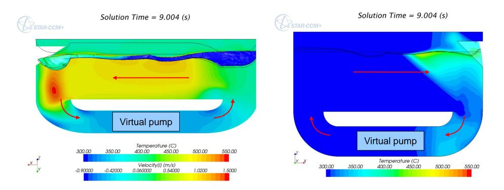
Increasing the flow rate to 39.0l/s, the velocity in the spallation zone reaches ~0.8m/s, the max. temperature is 451 C but the free surface becomes slightly unstable
