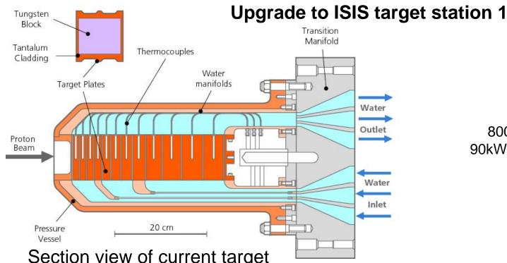
800MeV, 160kW, 50Hz 90kW heat removed in water
