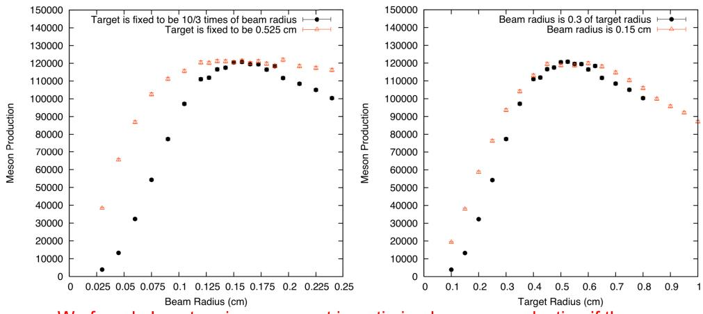
We found almost no improvement in optimized meson production if the beam radius is not fixed at 30% of target radius and optimized separately!
