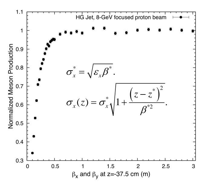
Relative normalized meson production is 0.84 of max at  $\beta^*$  of 0.3 m for  $\epsilon_x = \epsilon_y = 5 \ \mu m$ .
