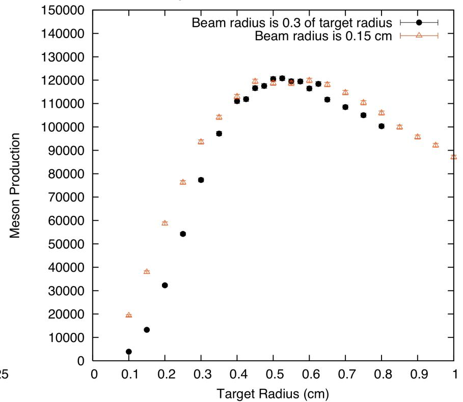
We found almost no improvement in optimized meson production if the beam radius is not fixed at 30% of target radius and optimized separately!
