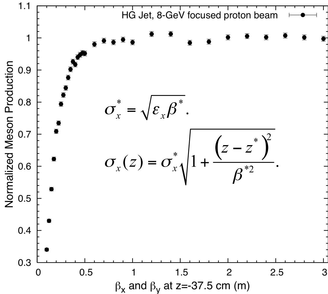
Relative normalized meson production is 0.84 of max at  $\beta^*$  of 0.3 m for  $\epsilon_x = \epsilon_y = 5 \mu\text{m}$ .
