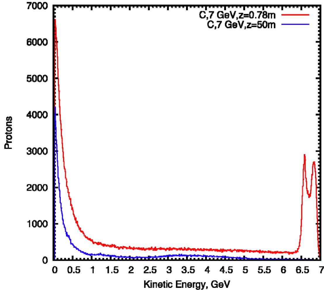
$z=0.78 \text{ m}$ :  $E(\text{total})=233739 \text{ GeV}$ ,  $E(\text{ave})=3.3396 \text{ GeV}$ ,  $\text{KE}(\text{ave})=2.4 \text{ GeV}$
