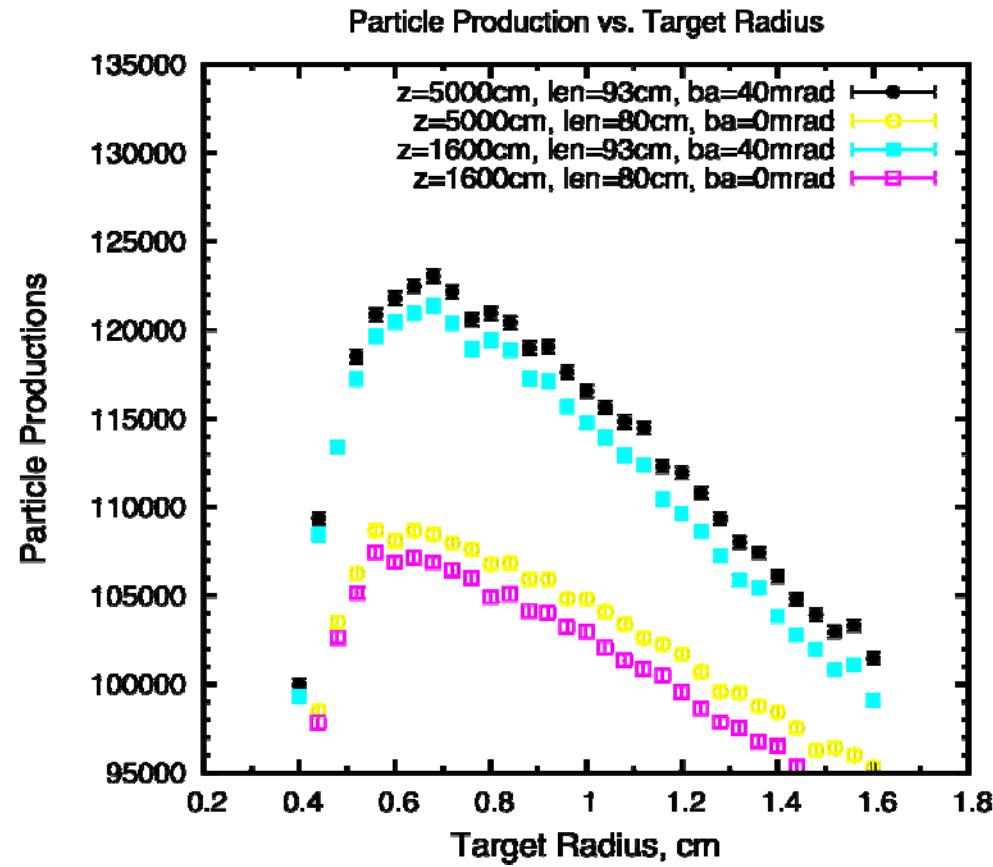
Optimized target length is 80 cm and target radius is 0.64 cm when beam angle is fixed at 0 mrad.
