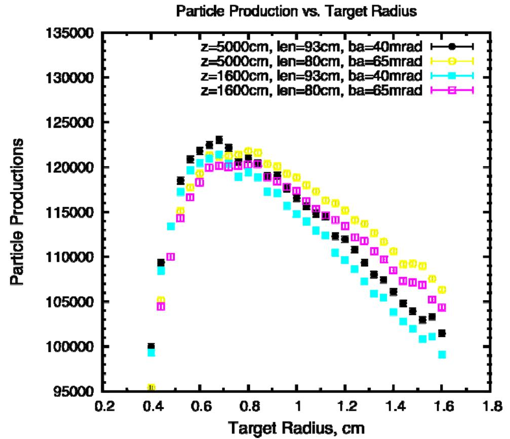
Optimized target length is 93 cm and target radius is 0.68 cm when beam angle is fixed at 40 mrad.
