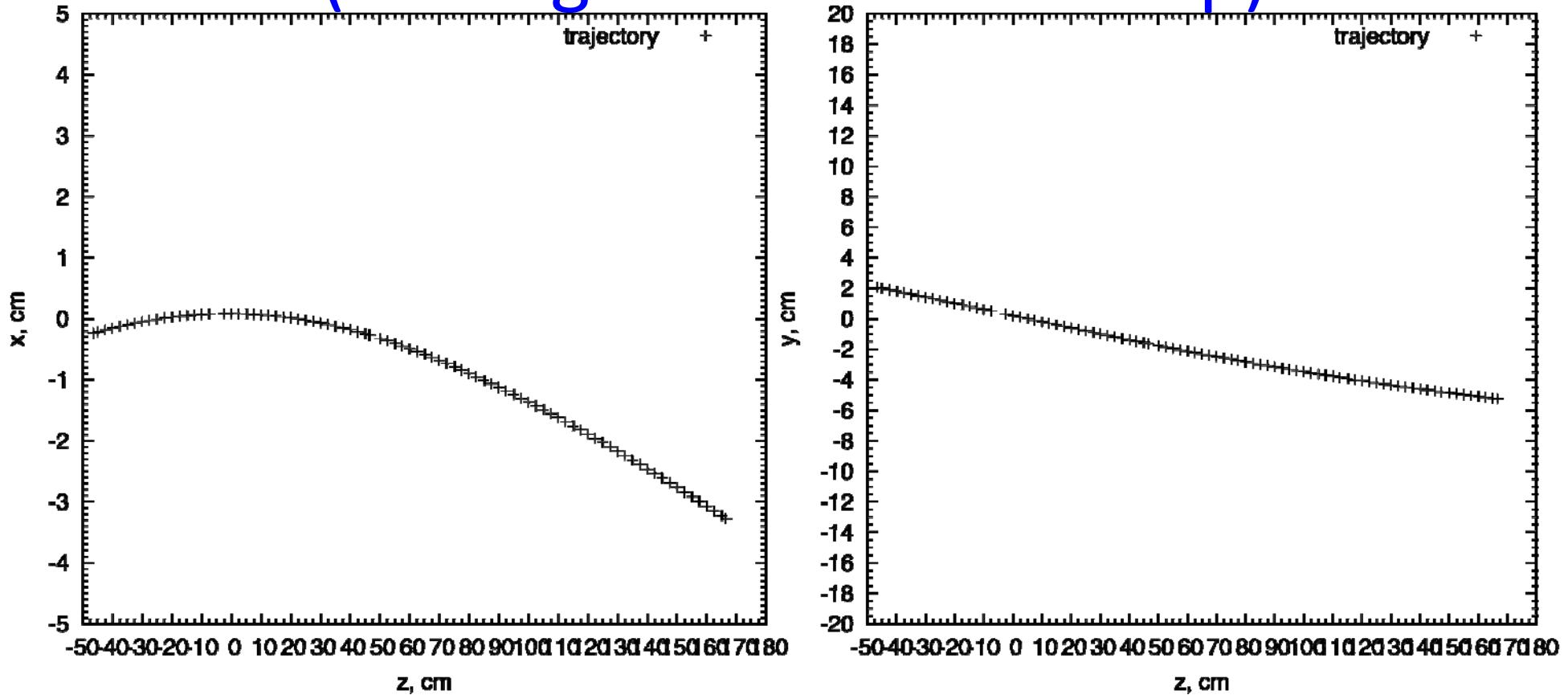
Target length: 93 cm, Target radius: 0.68 cm, Beam angle: 40 mrad
