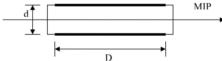
Fig. 10.19: Configuration with the metallizations of the diamond sensor parallel to the MIP trajectory. D is the maximum length of the metallization (in the case of a round metallization this distance would be the diameter).
