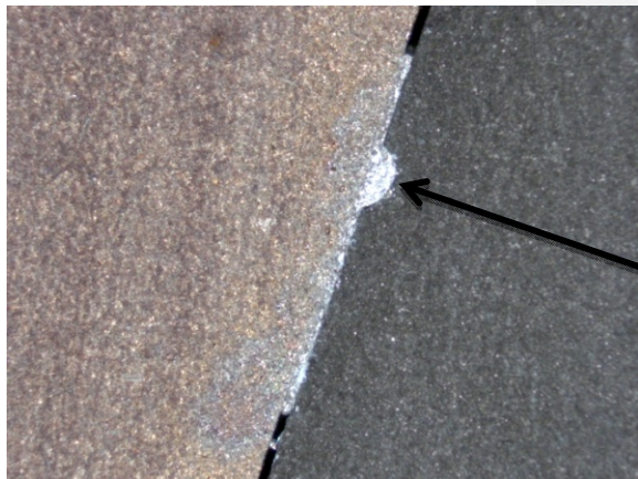
Aluminium intermediate layer, bonding temperature 550°C Soft aluminium layer reduces residual thermal stresses in the graphite
