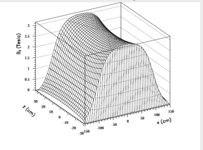
Figure 2: The z-component of the magnetic field in M1, plotted as a function of x and z. The x-direction is parallel to the beam, while z-direction is transverse to the beam.
