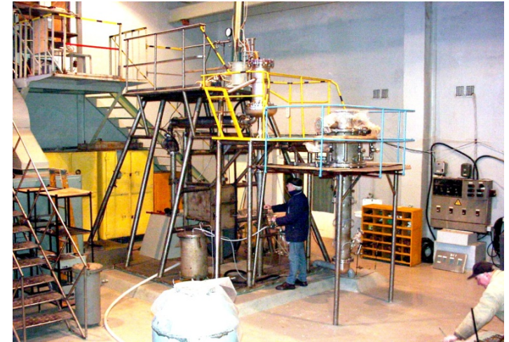
Existing Hg – loop in Institute of Physics (under reconstruction)(parameters of EMP p=4 bars; Q\sim 12l/s )
