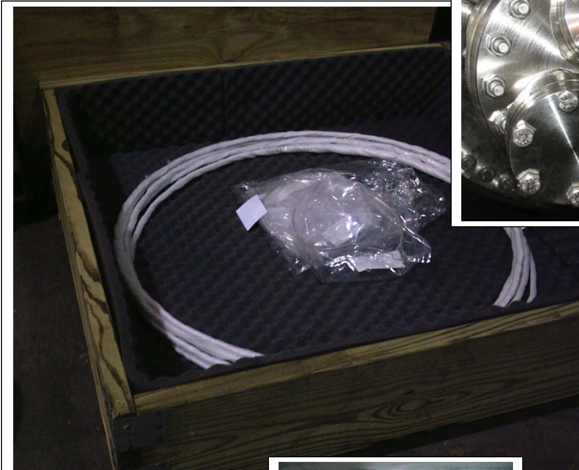
Metallic seals for the cover flange
