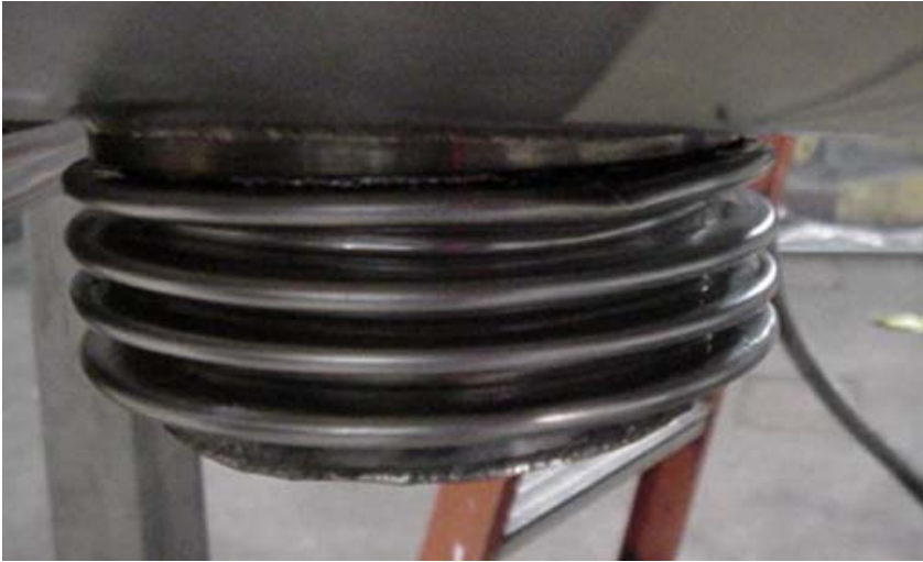
Centered bellows after repair attempt. – This one is being replaced. Damage is indicative of occurring with vacuum applied.
