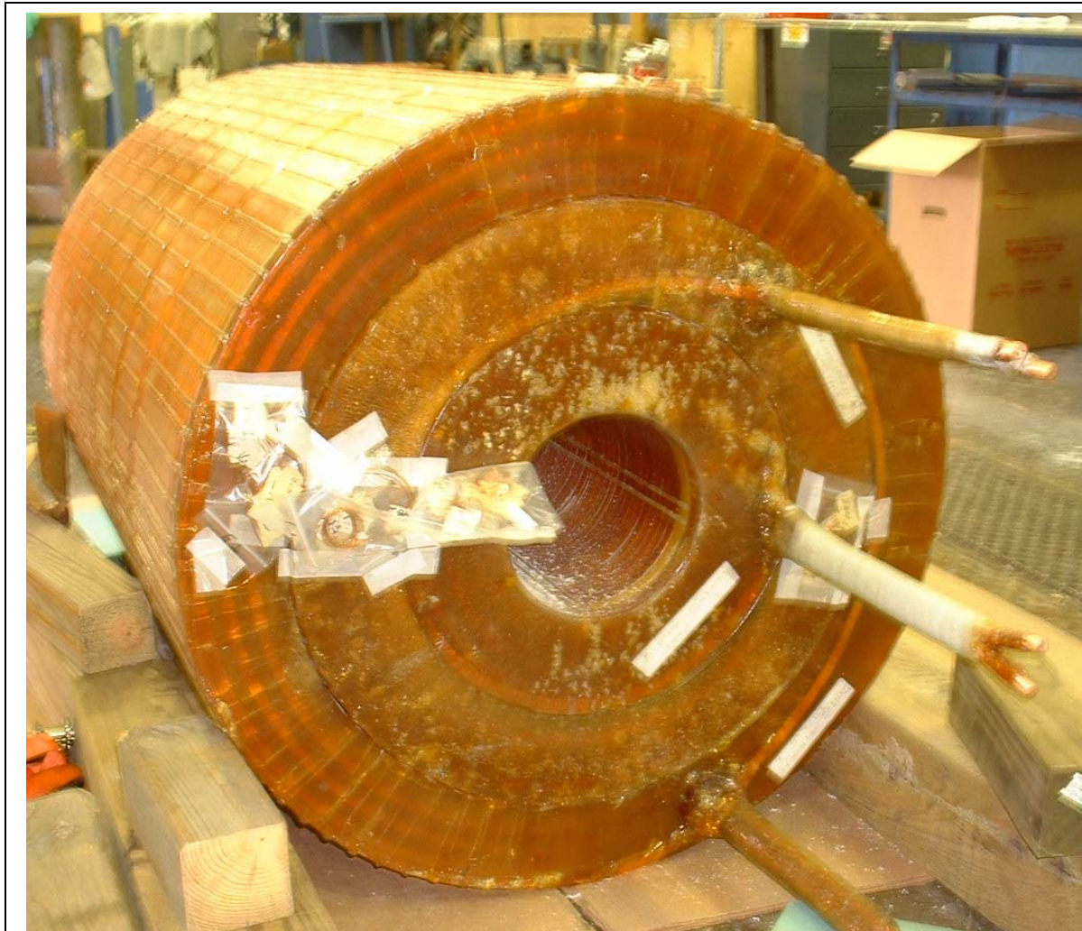
Leads threaded, Coils being prepared for shipping
