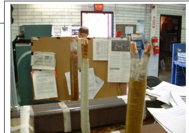
Leads threaded, Coils being prepared for shipping
