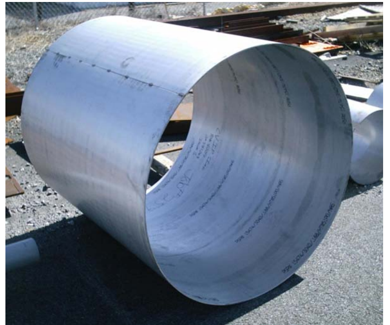
Outer Vacuum Shell at CVIP
