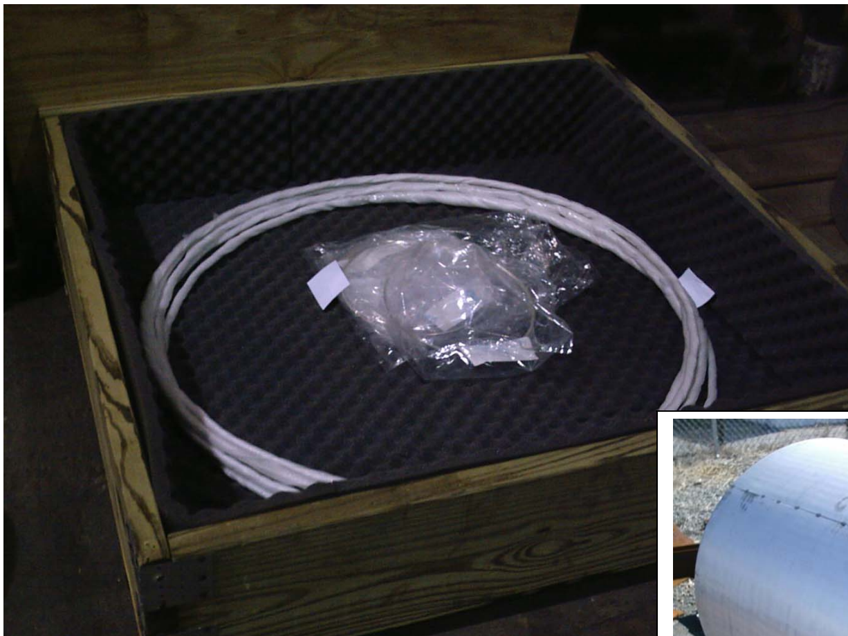
Metallic seals for the cover flange
