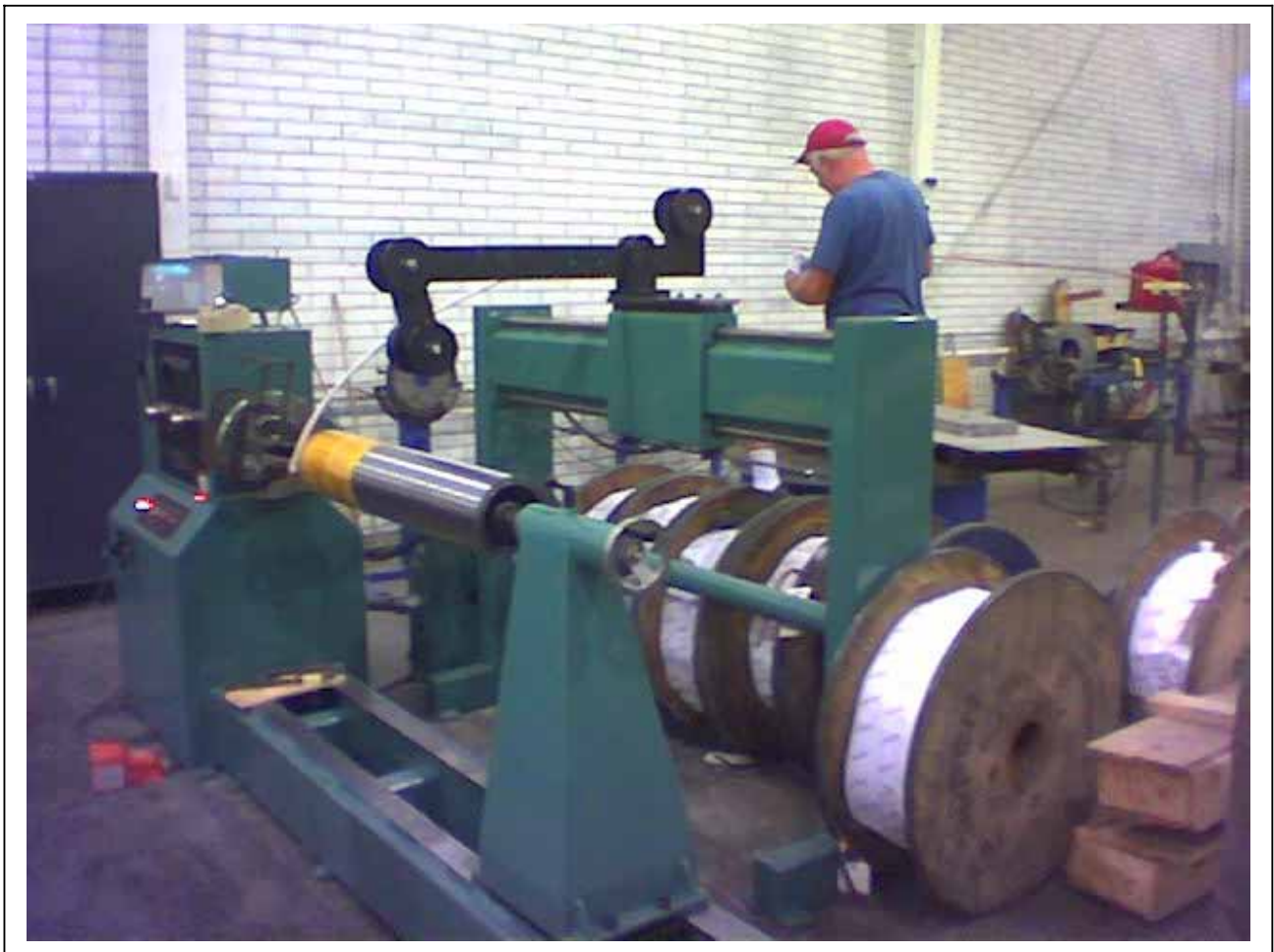
This was a test winding done by Everson before material purchase, and before the final pricing proposal to CVIP
