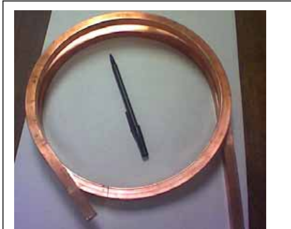
This was a test winding done by Everson before material purchase, and before the final pricing proposal to CVIP
