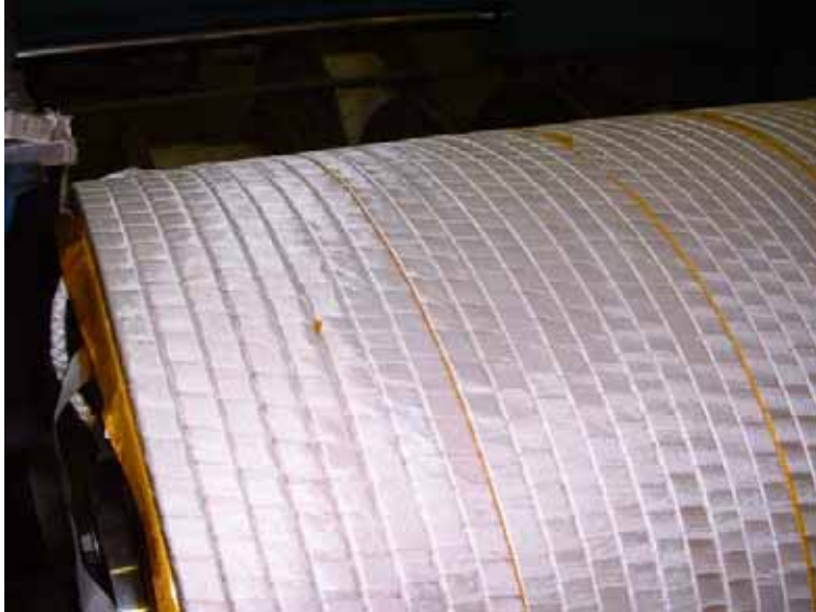
Photo taken by Dave Rakos at Everson 09-08-04. Kapton layer spaced at every eighth turn relieves axial tension in the layers near the cooling channels.
