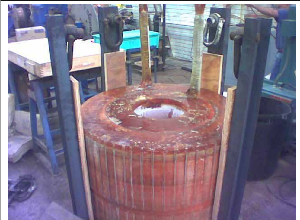
Successfully nested coils – Segment 1 in Segment 2
