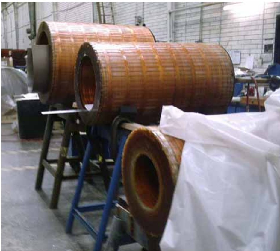
Segment #1 out of the mold. External Silicon fillers that form the “waffle” pattern have not yet been removed
