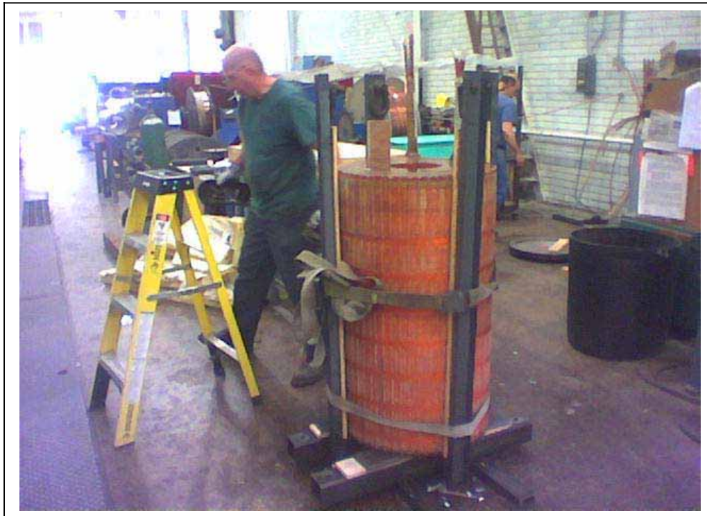
Successfully nested coils – Segment 1 in Segment 2
