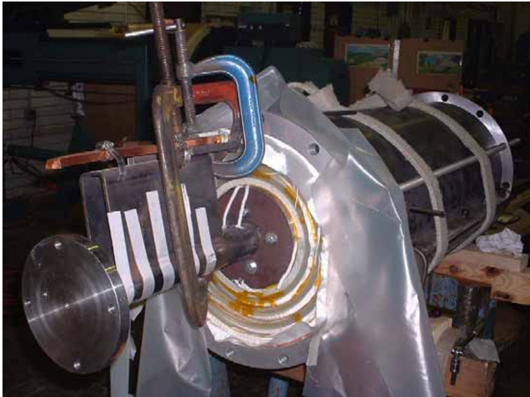
Segment 1 showing formed leads and portions of the mold
