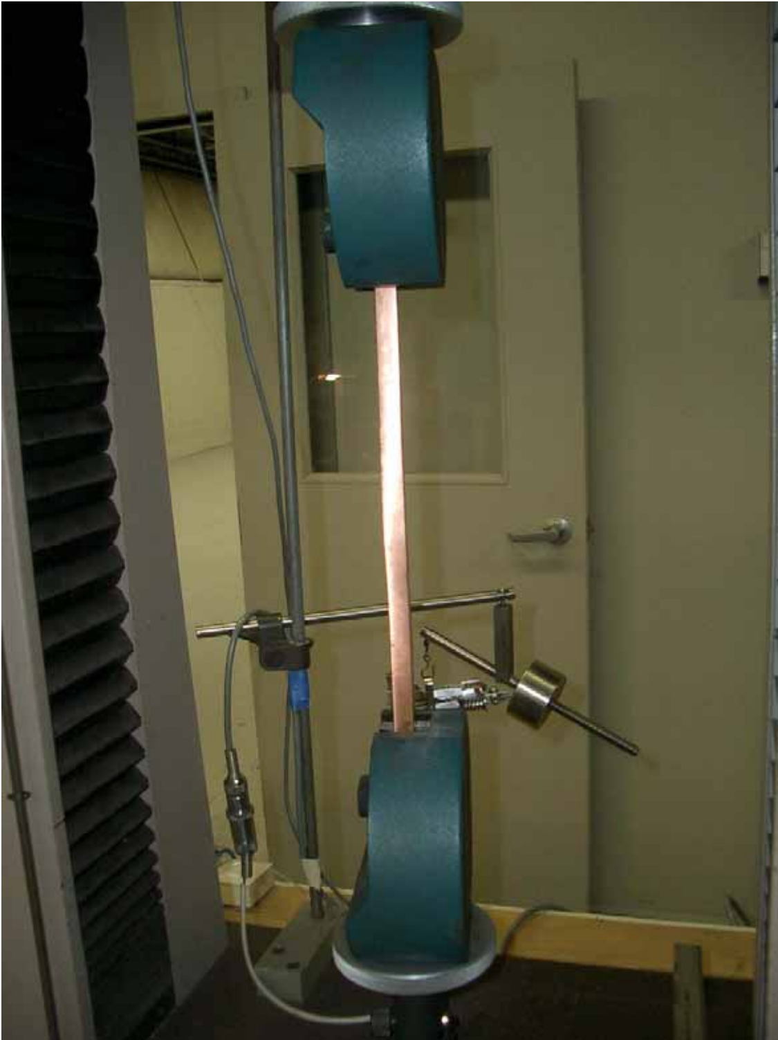
Silver Solder Joint Tensile Test
