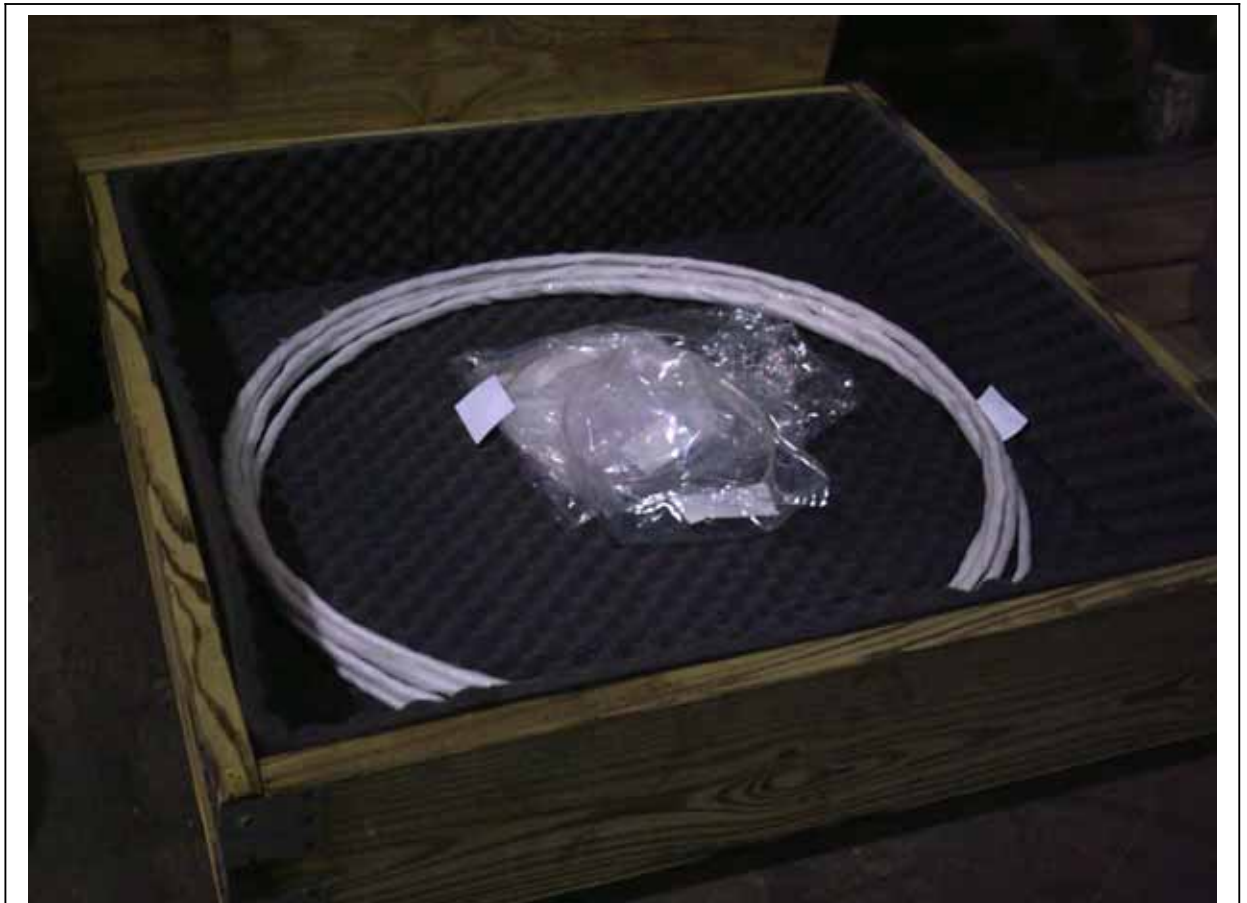
Metallic seals for the cover flange
