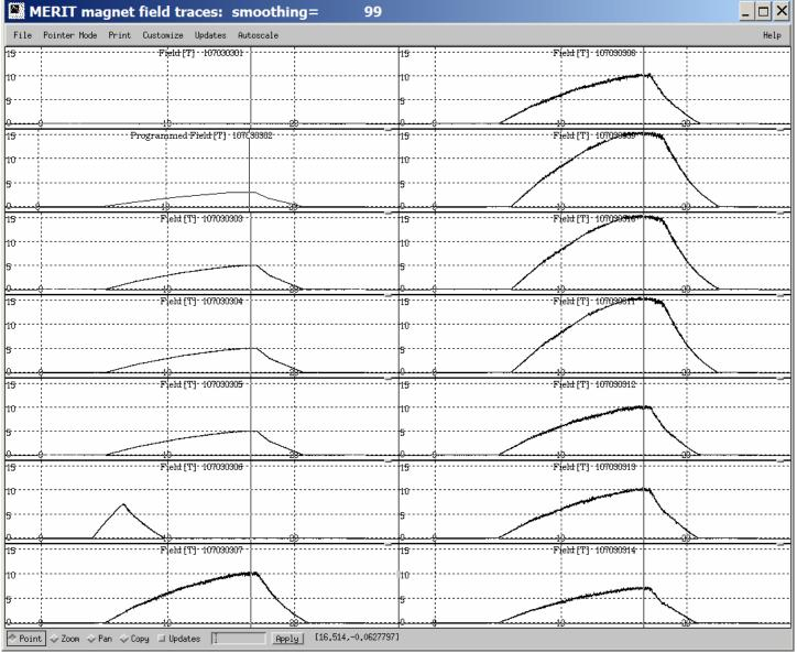
The trigger for the MERIT magnet pulses was generated at time zero for all traces. The recorded data for run 107030302 was somehow not stored, which accounts for the plot title "Programmed Field." The vertical line running through all traces shows the t = 16.5 s time point.
