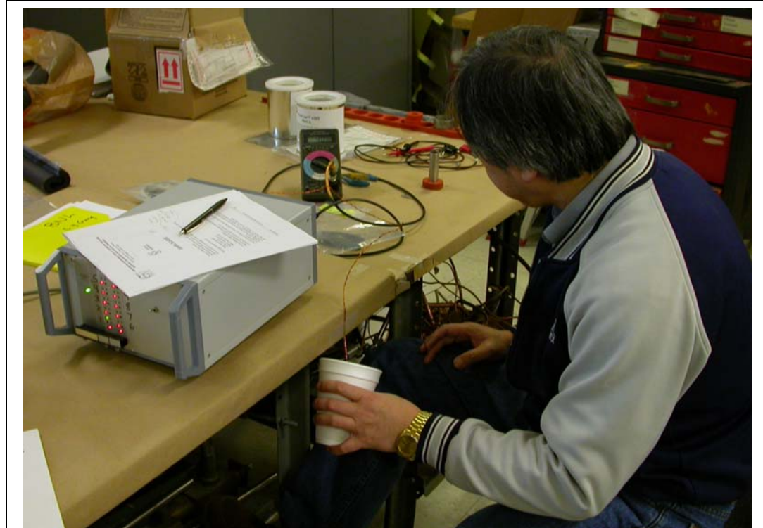
Feb 9 2006 test of the discrete level sensor – It did not seem to be able to detect when the diode was immersed or when it was in cold N2 gas just above the liquid. Voltage changed about 1mV out of 30 mV
