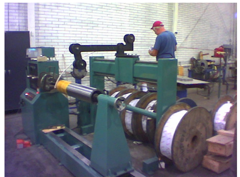
Winding Machine with the beginnings of segment #1
