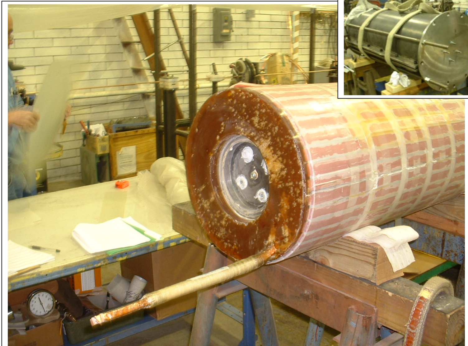
Segment #1 out of the mold. External Silicon fillers that form the “waffle” pattern have not yet been removed
