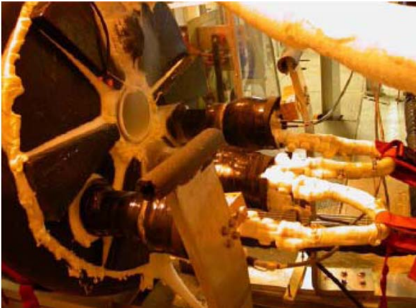
Thursday, March 30 2006 The cold end of the magnet. We had the bore heater off. Jumpers were not insulated.
