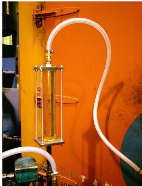
Epoxy fill site glass. Everson doesn't have a good method to measure the flow going into the coil
