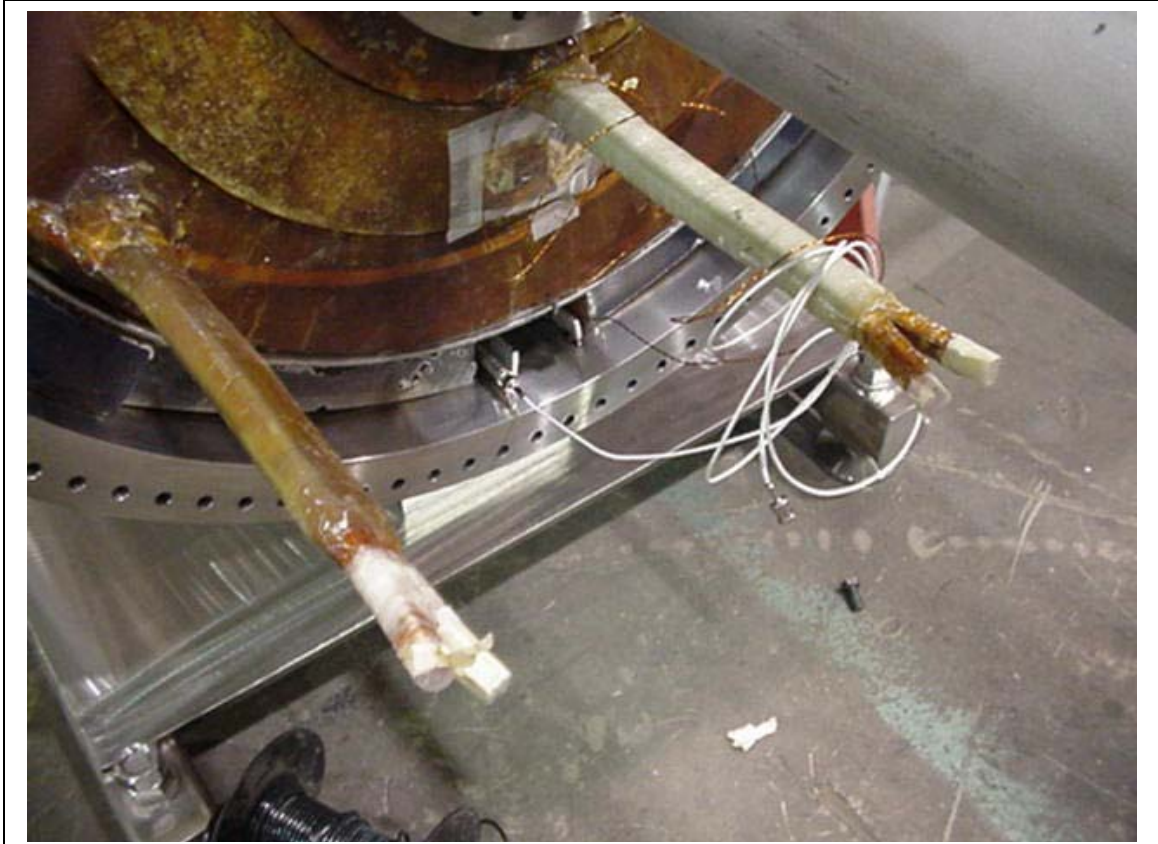
Lower capacitive level sensor, before the cover was closed.
