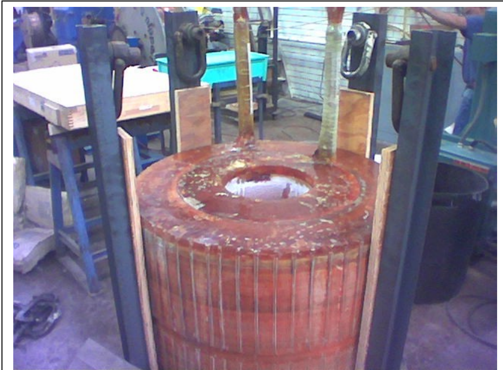
Successfully nested coils – Segment 1 in Segment 2
