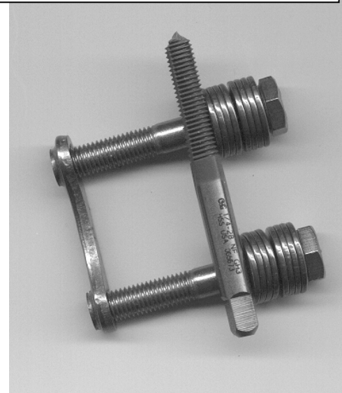
Platenut and Belleville stacks added to the packing nut/gland assembly
