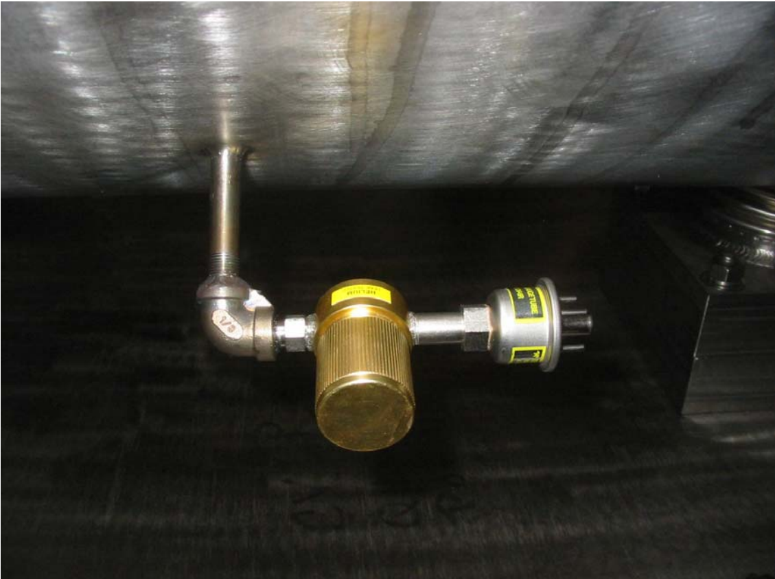
Thermocouple type or TC Vacuum Gauge supplied by CVIP. Only good below 2 Torr
