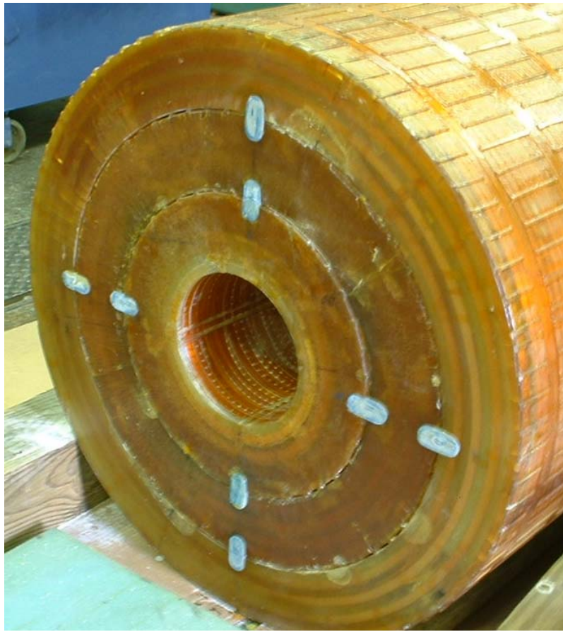
Tabs to maintain torsional registration
