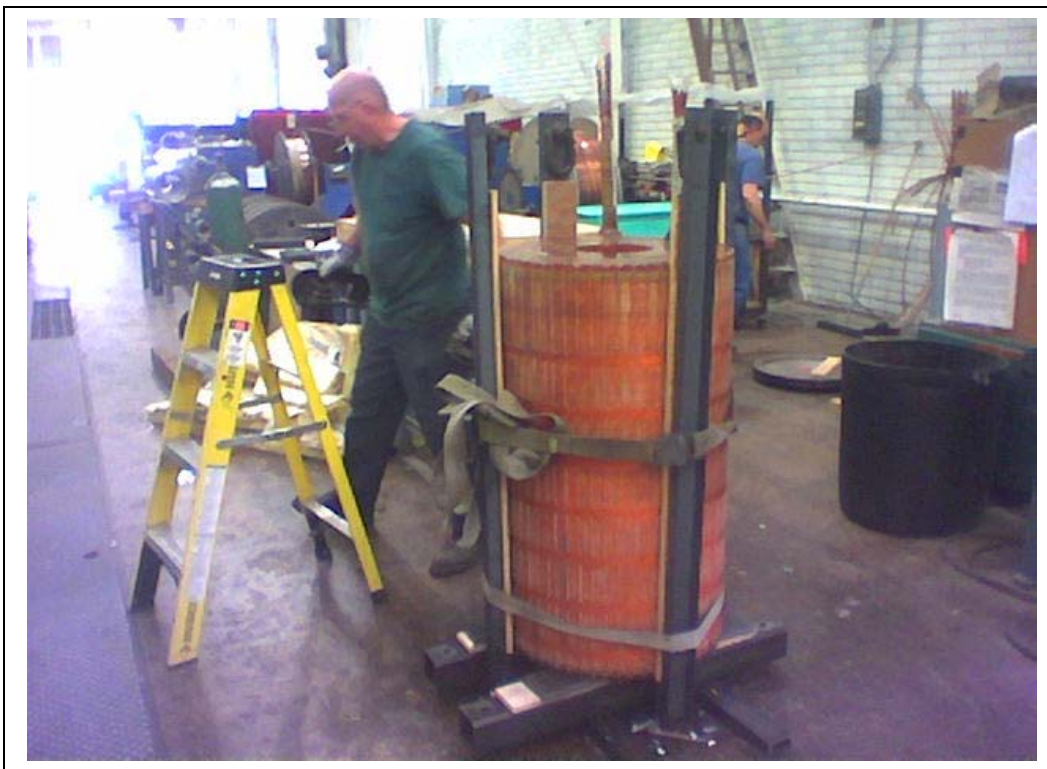
Successfully nested coils – Segment 1 in Segment 2
