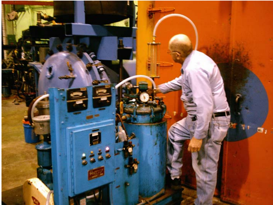
Lenny, an Everson Tech, watching the epoxy fill process A vacuum is maintained on the mold (inside the autoclave box) with a vacuum pump (not shown) to the right of the autoclave). The epoxy tank is at an atmosphere gage. Ron adjusts epoxy flow manually. After the mold is filled, pressure is cycled to drive off bubbles. The mold is under pressure during the cure cycle to minimize the remaining bubbles.
