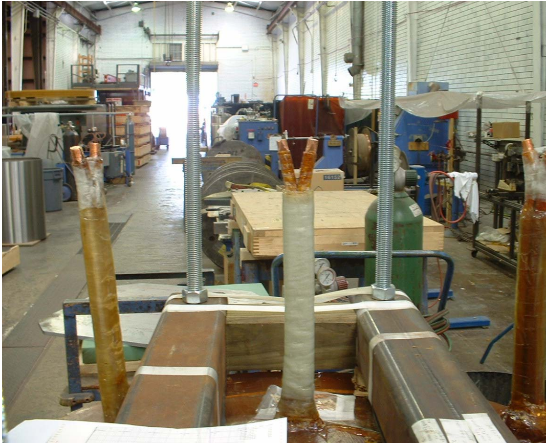
Leads threaded with the coils being prepared for shipping
