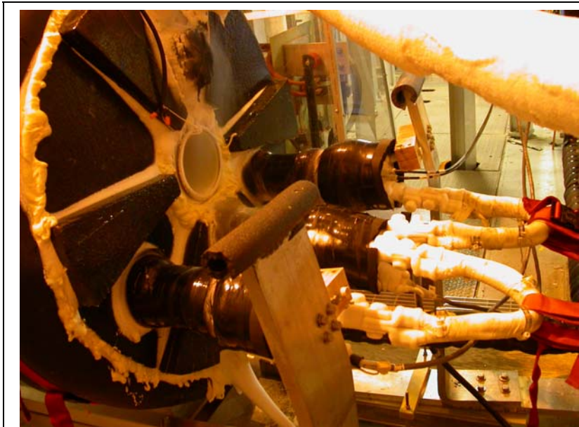
Thursday The cold end of the magnet. We had the bore heater off, Jumpers were not insulated.
