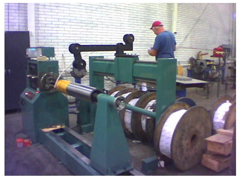
Winding Machine with the beginnings of segment #1
