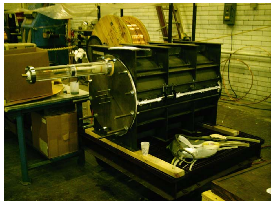
Segment #2 Mold (with Coil enclosed)
