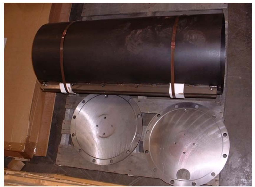
Coil Mold for Segment #1. Successfully used for its impregnation
