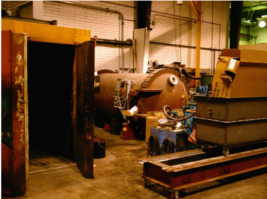
Everson autoclave (Box with Doors) Epoxy pumping equipment, and vacuum pumps) – Used for all three coil segments
