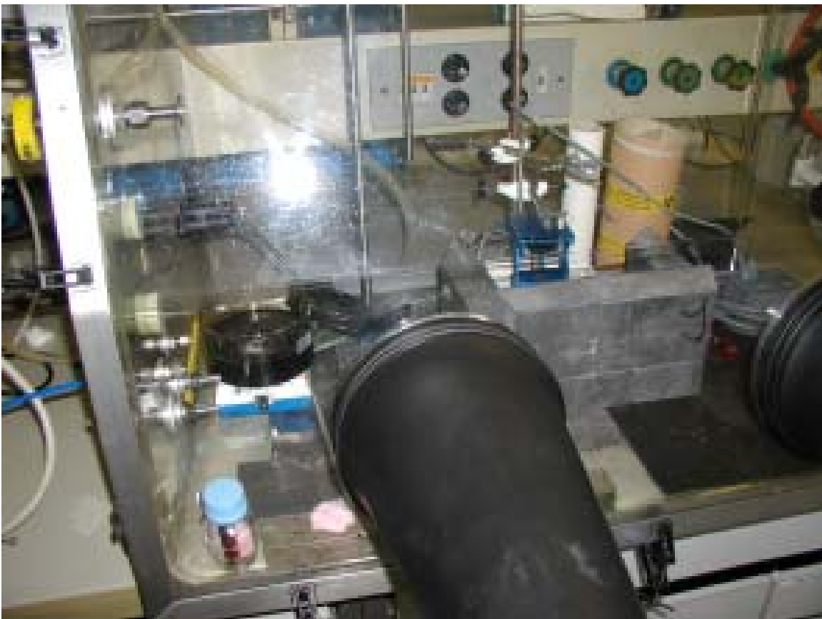
Figure 14: Glove box system. Top: outside view with gas pre-drying columns and oxygen sensor. Bottom: Inside view with lead shielding and oxygen absorber solution (left side).
