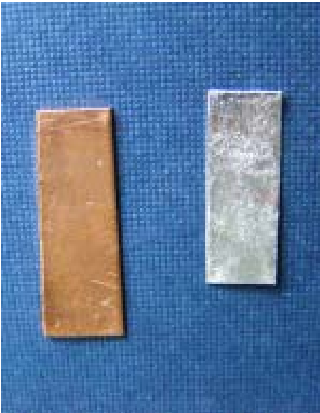
Figure 23: Untreated copper plate and copper plate amalgamated in a saturated aqueous \text{HgCl}_2 -solution, after mechanical cleaning of the surface.
