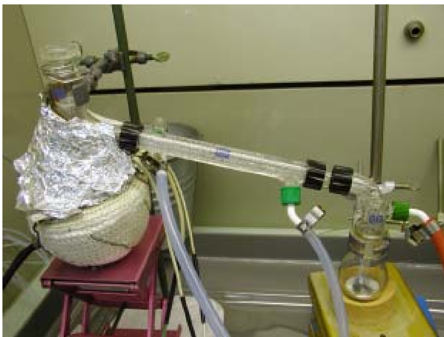
Figure 13: Apparatus used for the vacuum distillation of mercury prior to the preparation of radionuclide-doped mercury samples.
