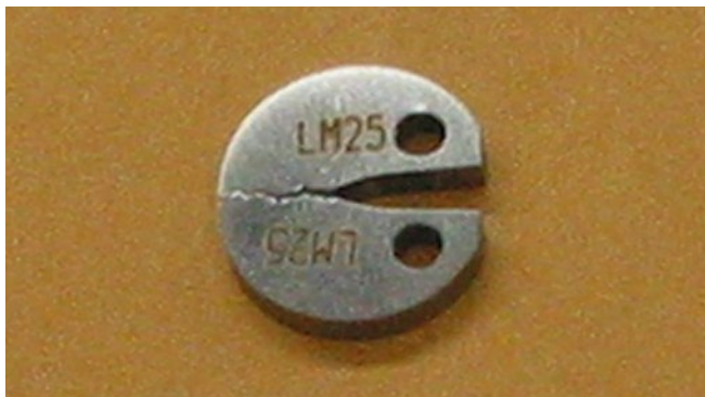
Brittle fracture of ferritic/martensitic steel fracture toughness specimen
