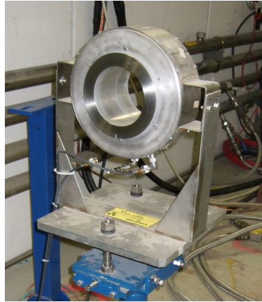
Figure 3.6. The TT2a current transformer.
