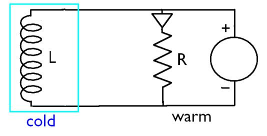
Now, when there is a quench, the rising resistance of the coil generates enough voltage to allow the diode to conduct the current through the external resistor. The introduction of the resistance generates a voltage across the coil that brings the current down faster than in the cold diode case. Now some fraction of the stored energy is dissipated in the external resistor, thus reducing temperature rise in the coil.
