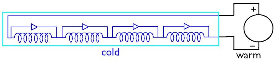
Now, when one coil quenches, a voltage develops that shorts the current through the diode. The magnet that quenches must absorb its own energy, but the other magnets can continue to carry current that, because it does not flow through the quenched coil, does not dump their energy in the quenched coil. In due course the power supply is turned off to bring down the other magnets in a safe way. This is done in RHIC and, I think, in the LHC.
