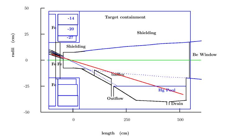
Fig c shows the containment within the superconduction coils. Note that sc coil 2 has been moved out  $5\mathrm{cm}$  and the following coils moved in by the same amount.
