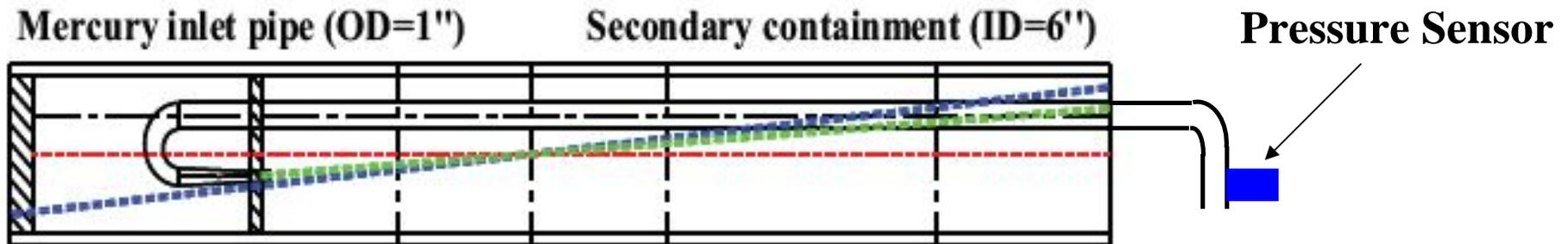
Green, Mercury jet at 33 mrad to magnet axis      Red, Magnet axis
