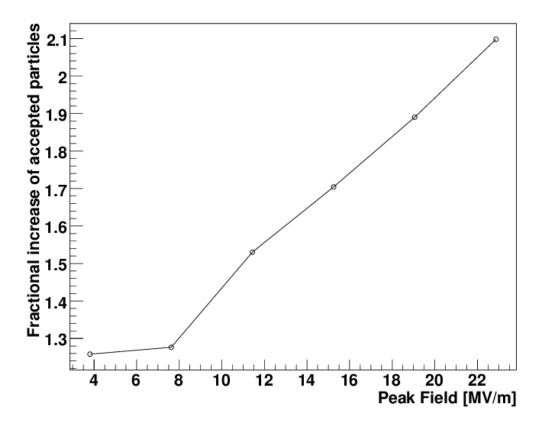
FIG. 6. Degradation in cooling performance with decreased RF voltage. The baseline cooling lattice was simulated with Lithium Hydride thickness proportional to RF peak voltage to account for the reduction in energy gain and the good muon yield was calculated.
