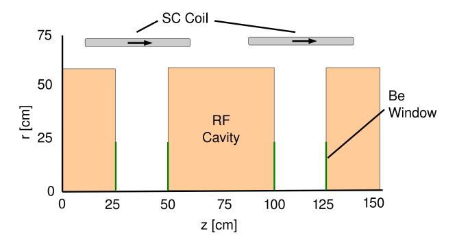
FIG. 3. Schematic radial cross section of a rotator cell.
