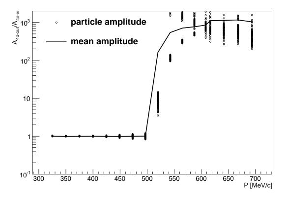
FIG. 1. (top) x-y projection and (bottom) fractional change in transverse amplitude of a shell of muons after transport through the chicane system for a variety of momenta. The muons were created on the surface of a hyperellipsoid in  $(x, p_x, y, p_y)$  space at intervals of 25 MeV/c total momentum. The surface was chosen at each momentum to be constant in the 1.5 T field with 4D transverse amplitude of 50 mm. Simulation in MAUS 0.3.1.
