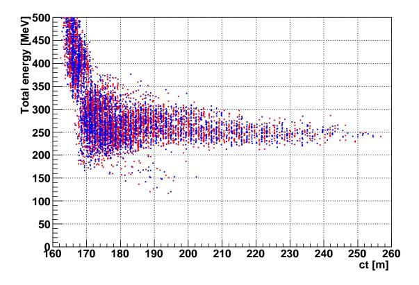
FIG. 5. Distribution of particles in longitudinal phase-space at the phase rotation end.  $\mu+$  are shown in red and  $\mu-$  are shown in blue.
