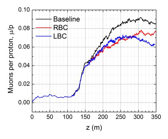
FIG. 7. Simulated good muon yield with different bucked coil lattices. The bucked coils were used also in the phase rotation section in these simulations.
