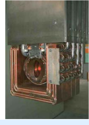
COLLIMATOR 2 & 3 Beam losses: 22/18 %
