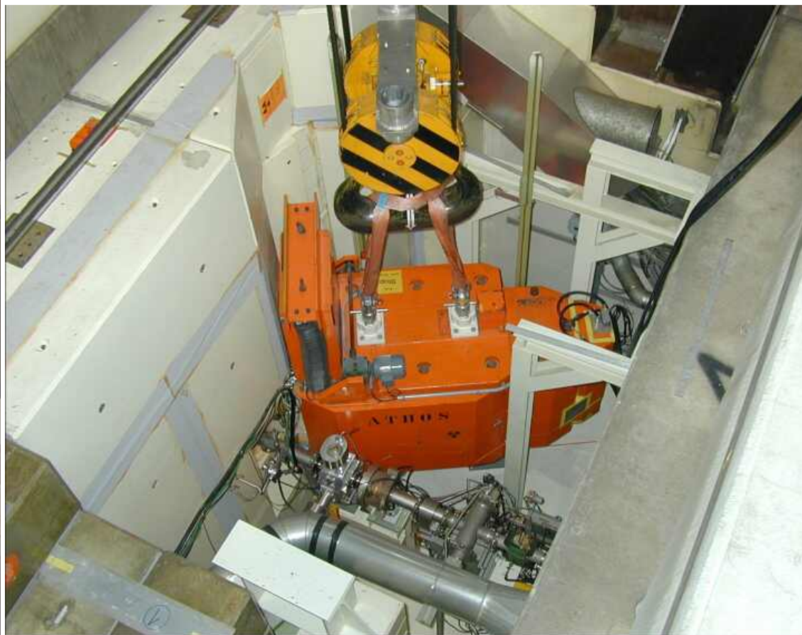
Operation of the remotely controlled shielded flask
