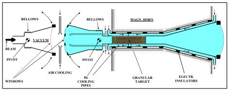
Figure 1: The granular, stationary target, its He-gas cooling system and its pivoting windows integrated into the magnetic horn-pion-collector.
