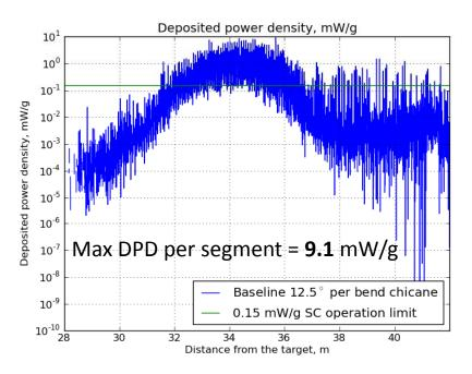
At the same time, certain coil segments can get up to 9.1 mW/g (3 longitudinal, 2 radial, 12 azimuthal segments per coil) due to the non-uniformity of energy deposition.
