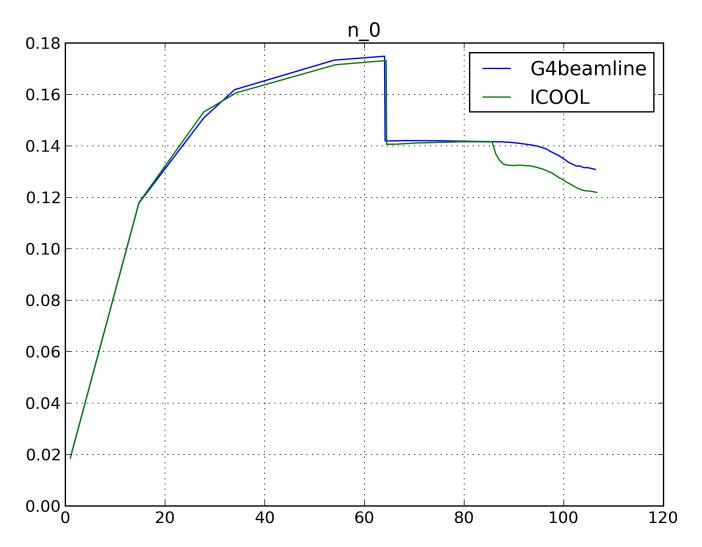
Weird particle loss at the beginning of buncher in ICOOL. Not resolved yet.
