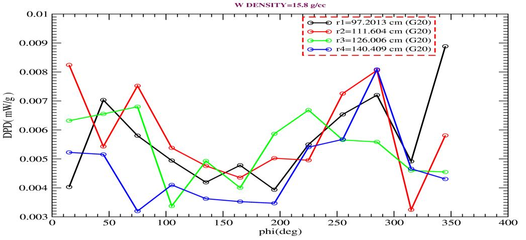
AS WAS EXPECTED 20 cm OR LARGER GAPS IN THE SHIELDING FOR THE CRYOSTATS #1 AND #2 APPEAR TO PRESENT NO PROBLEM FOR THE PEAK DPD IN SC#4, IT IS MUCH LOWER THAN THE ITER LIMIT. PEAK VALUES FOR P12 APPEAR IN THE LOWER HALF OF THE COIL (DUE TO Hg POOL).
