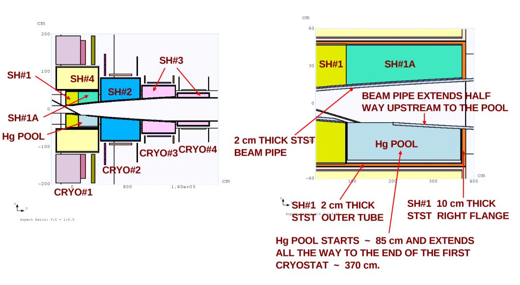
SHVS WALLS, Hg POOL VESSEL DOUBLE WALLS, Be WINDOW, He GAP IN BE WINDOW AND IN HG POOL HAVE NOMINAL VALUES FOR THEIR THIKNESS. STRESS FORCES ANALYSIS AND LOCAL DPD DISTRIBUTION WILL BE USED TO DETERMINE THEIR VALUES.
