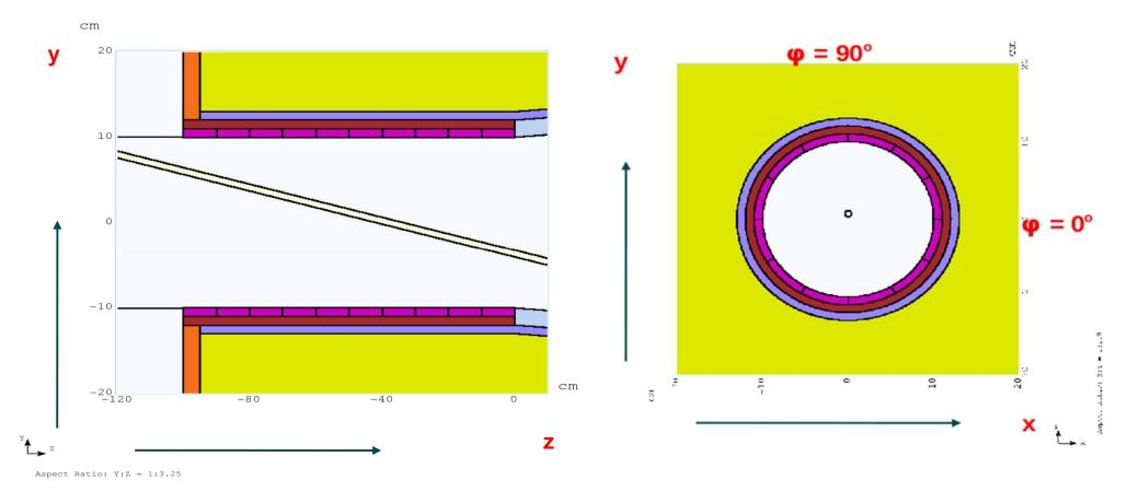
$\begin{array}{ccccccc} 10.0 < r < 11.0 \ cm & dr = \ 1.0 \ cm & N_r = \ 1 \ bins \\ - \ 100.0 < z < 0.0 \ cm & dz = \ 10.0 \ cm & N_z = \ 10 \ bins \\ 0.0 < \phi < \ 360.0 \ deg. & d\phi = \ 30 \ deg. & N_\phi = \ 12 \ bins \\ N_{tot} = \ 120 \ "pieces" \end{array}$
