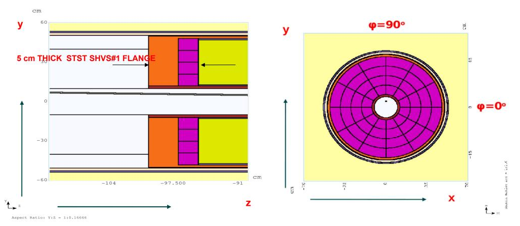
ONLY THE FIRST (INNER) 2 cm OF THE FLANGE VOLUME OF THE SHVS#1 WAS SEGMENTED.
