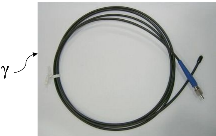
2 meter long, 1-mm diameter blue emission scintillating fiber
