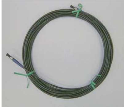
2 meter long, 1-mm diameter blue emission scintillating fiber
