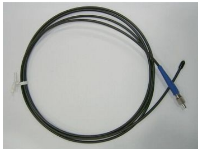
2 meter long, 1-mm diameter blue emission scintillating fiber
