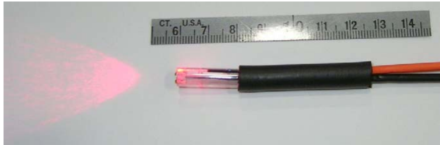
d=0.5 mm sapphire ball lens, increase the NA of illumination to \Phi \sim 45 degree
