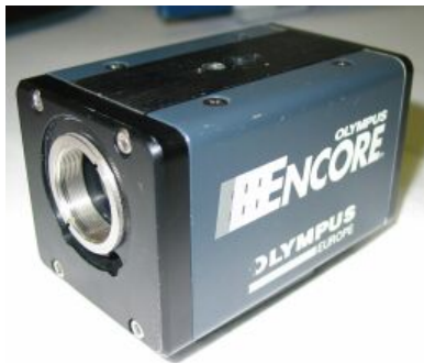
Olympus Encore Camera 2 ms frame rate 100 \mu s exposure
