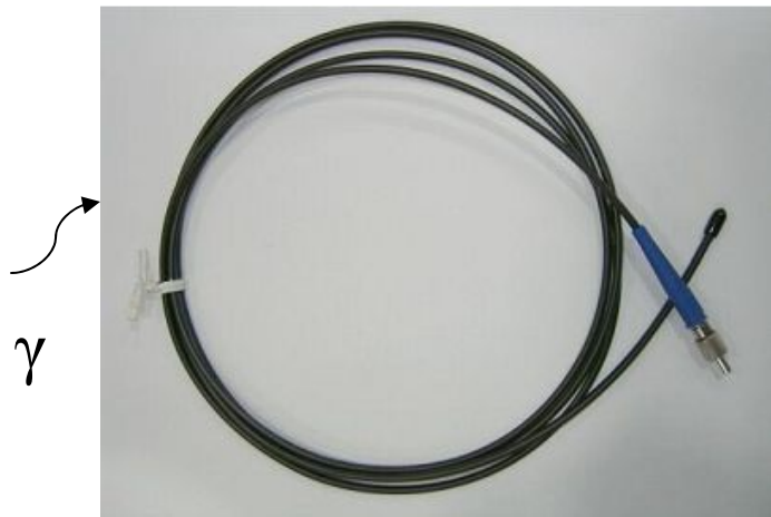
2 meter long, 1-mm diameter blue emission scintillating fiber
