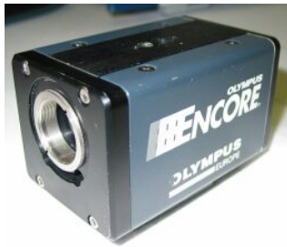
Viewport 4, Olympus 0.5 ms frame rate 33 \mu s exposure 160x140 pixels
