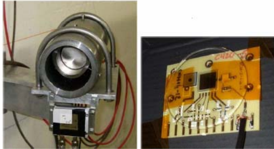
Fig. 4. Left: photo showing one detector assembly: the ACEM detector is located at the top with the pCVD diamond box at the bottom. Right: the board housing the pCVD diamond detector (center) and a pin diode (top left).
