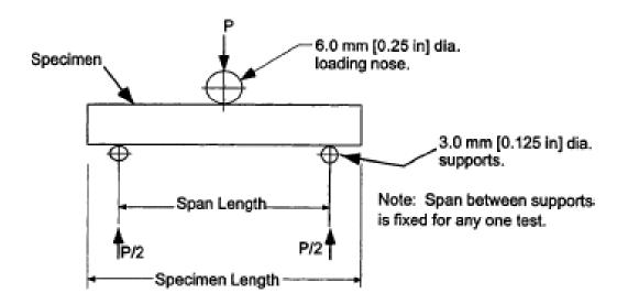
length 6 x thickness, span 4 x thickness and width 2 x thickness Recommended thickness =4mm
