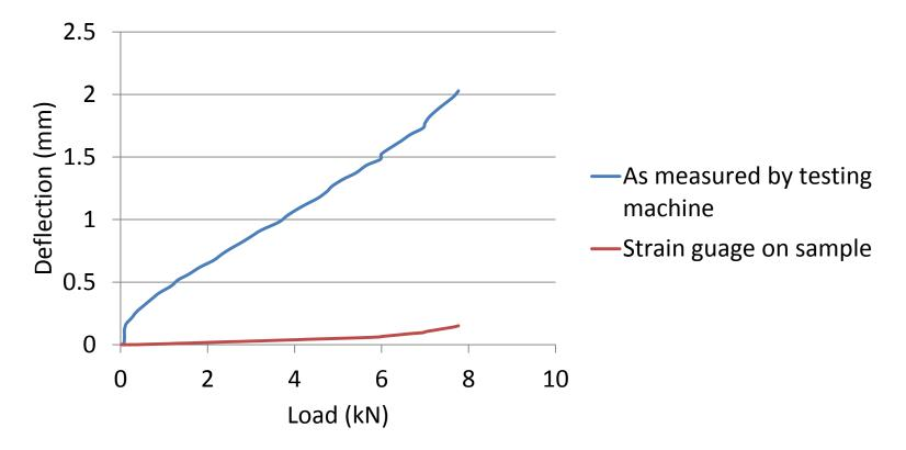
If interested in modulus it is critical to measure movement of sample not overall movement of testing machine
