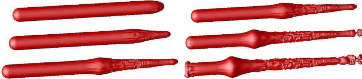
Figure 3.9: Disruption of a mercury jet on entering and exiting a solenoid magnet, as simulated by the FronTier code.
