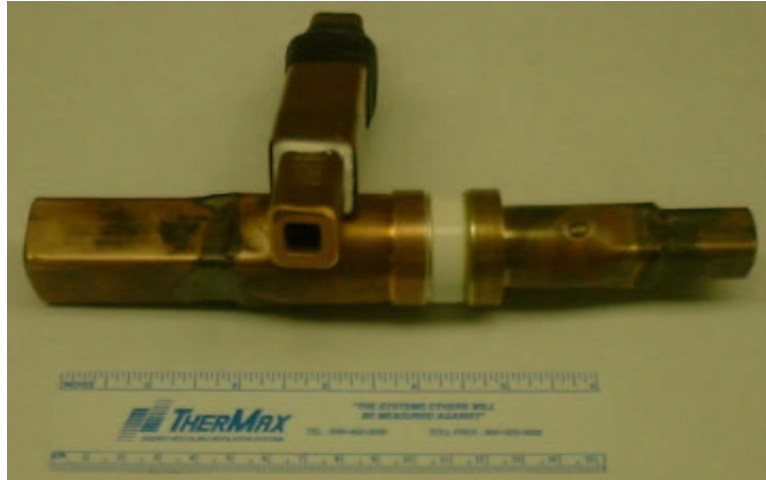
Figure 3.26: Mineral-insulated hollow conductor developed for Japan Hadron Facility. The end-on view shows the white layer of powdered MgO insulation sandwiched between the copper hollow conductor and its sheath, also of copper. Of the cross section, 17% is cooling passage, 37% conductor, 28% insulation and 18% sheath. The side view shows a conductor termination, brazed of several parts that confine the MgO and hold the glossy white ceramic ring that keeps the sheath isolated from the current-carrying conductor.
