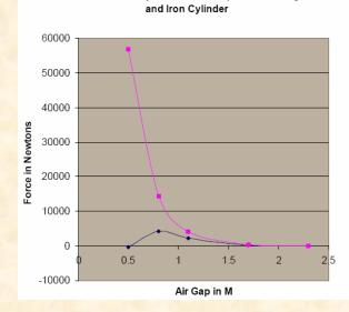
Force on 416 Lb Cylinder vs. Air Gap between Magnet
